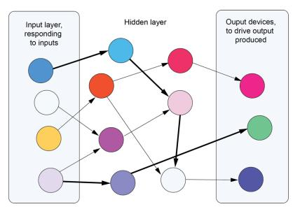
Neural networks were designed to mimic the processing inside the human brain. They consist of a series of interconnected nodes (artificial neurones). Each neurone can accept a binary input signal and potentially output another signal to connected nodes.
