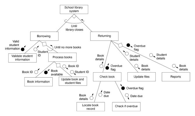
Further detail for each of the lower-level subroutines can be shown in a separate structure chart, using the same name as the subroutine used in the main structure chart.
