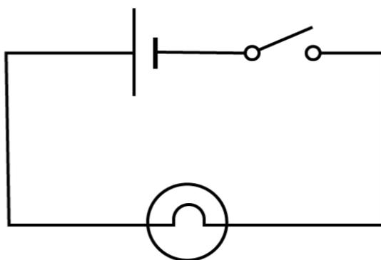
This diagram shows a complete circuit with an electrochemical cell, an open switch and a light globe connected by a conductor wire.
